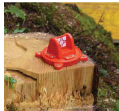
Example of the use of RS193rM as a fixed point on different surfaces and for the exact alignment of the drill carriage.
