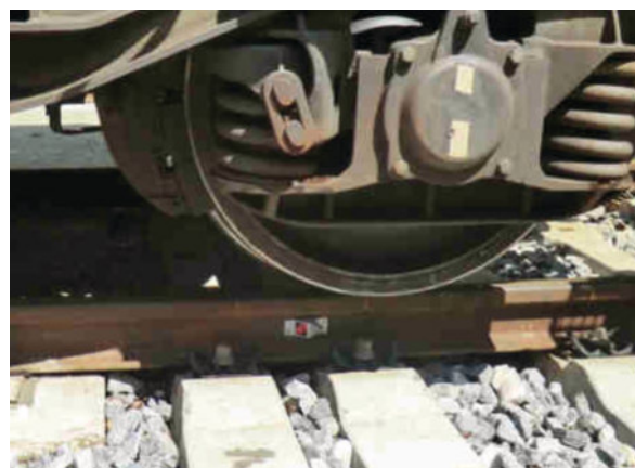
RSM P15 for measurements with Robotic total station during the loading.
