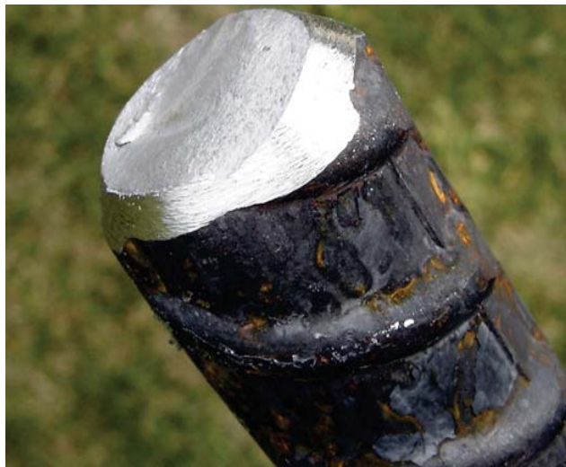
Rebar with bevelled end
