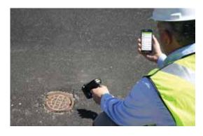
Field Data Collection with InfraMarker's Mobile Application, certified readers and locators find marked assets quickly and efficiently.
