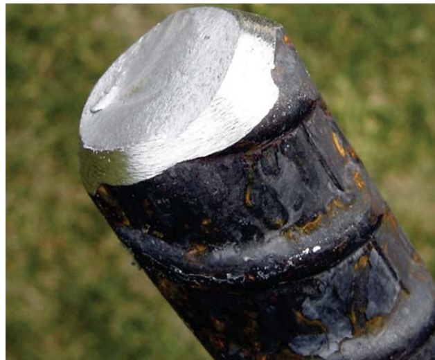
Rebar with bevelled end
